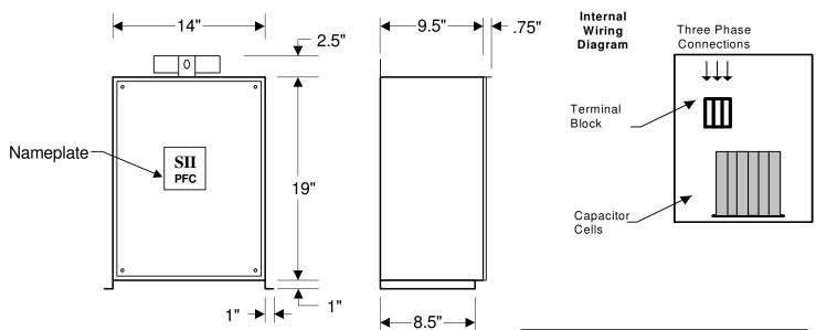
MODEL M036.0-480-NF 36 KVAR 480 VOLT Non Fused Three Phase 60 Hz NEMA 3R Enclosure Rated Current: 43.2 Amps Recommended Wire Size: 6 AWG APPROX. WEIGHT 42 LBS. EACH
